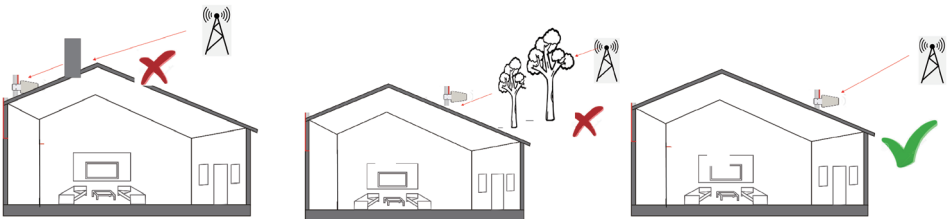
Figure 3 — Aim the outdoor antenna toward the nearest cell tower.
