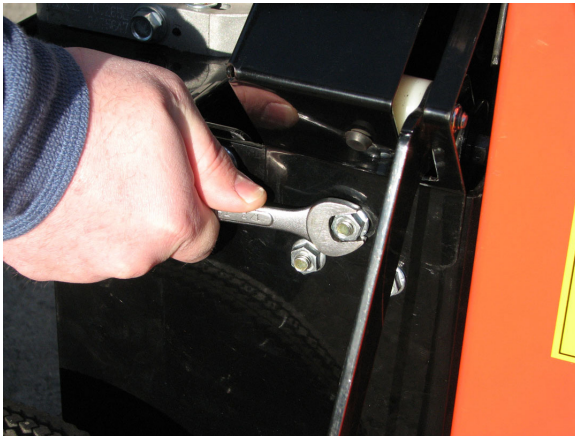
Figure 5.10 Belt Shield Removal
