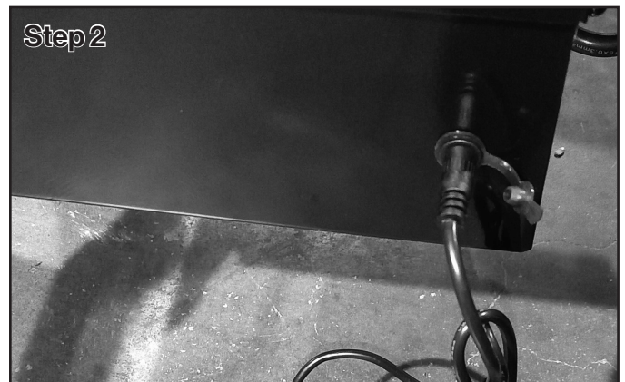
Insert the charger into the battery charging port.
