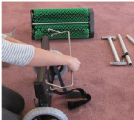
8. Insert front Bar on from of Transport Trolley
