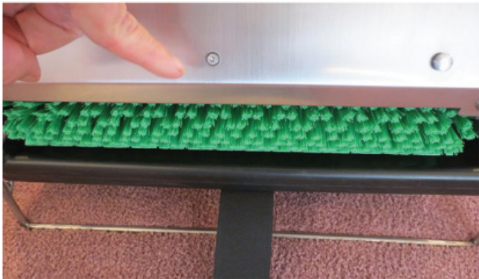
15. Removing Dust Cover – Push Button & Slide Left
