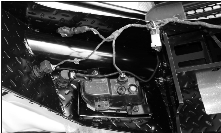
(Fig 17) Use the included (2) Wire Harness Extensions as necessary to reach the parking sensors
