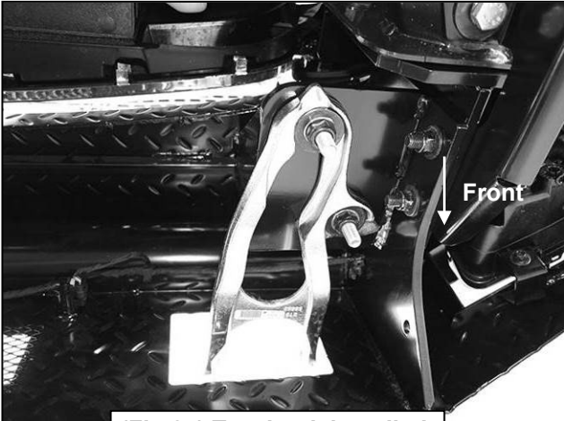
(Fig 25) Tow hook installed
