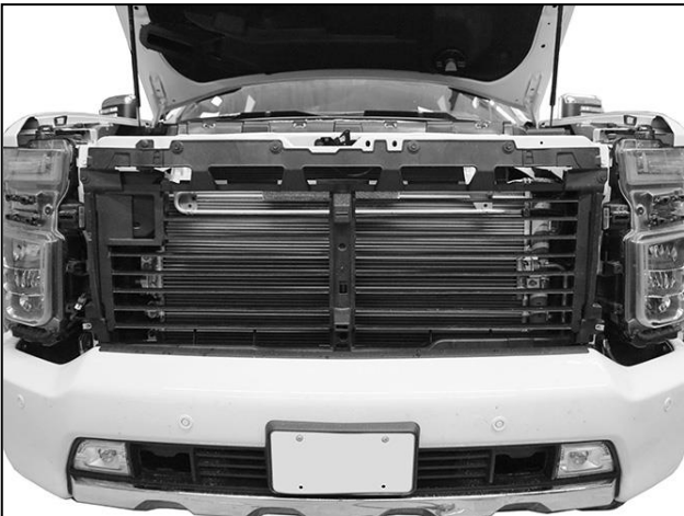
(Fig 7) Grille and fascia removed
