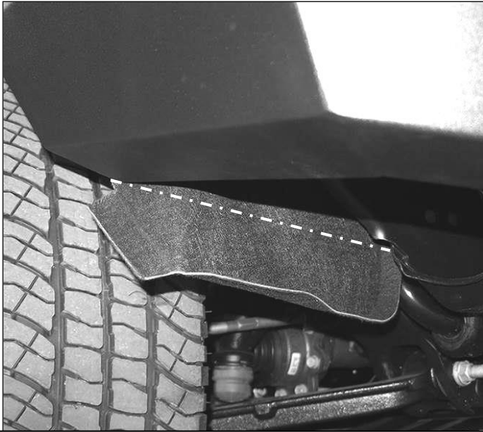
(Fig 26) Trim fender liner flush with bottom of bumper
