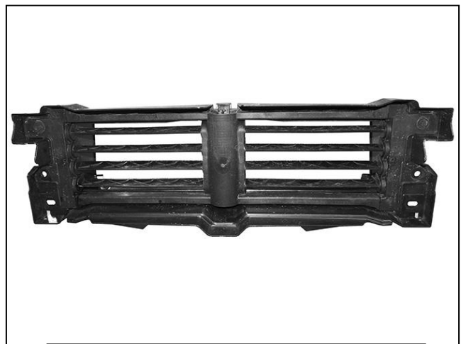
(Fig 19) Remove inner shutter assembly from plastic outer housing (if equipped)
