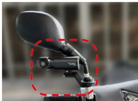
Right side (outer) installation.
