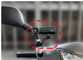
Right side (inner) installation.
