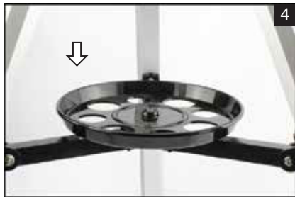
4 Place the (N) accessory tray on top of (O) center leg brace. Thread the (N) accessory tray into the threaded hole in the center of the (O) leg brace and screw into place.
