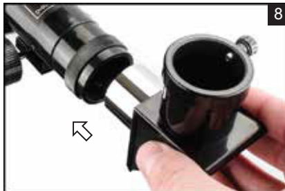
8 Insert the chrome barrel of the (C) diagonal into the focuser tube on the (L) main telescope optical tube and tighten the set screw.
