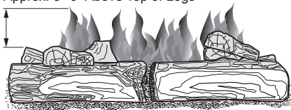
Figure 31 - Correct Burner Flame Pattern
