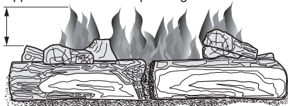
Figure 23 - Correct Burner Flame Pattern
