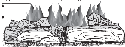
Figure 32 - Correct Burner Flame Pattern Actual logs will vary from those shown
