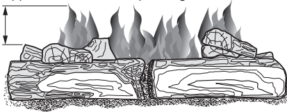
Figure 32 - Correct Burner Flame Pattern
