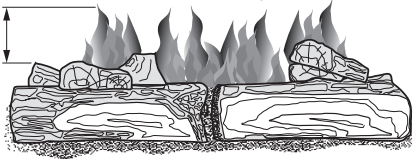
Figure 24 - Correct Burner Flame Pattern with Control Knob Set to HI (5)
