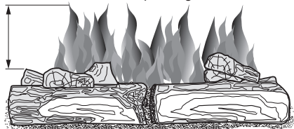
Figure 21 - Incorrect Burner Flame Pattern
