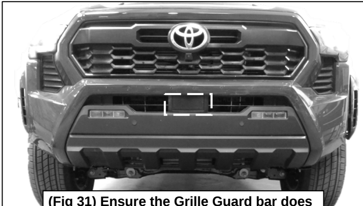
(Fig 31) Ensure the Grille Guard bar does not block or interfere with the Adaptive Cruise Control Sensor (white box)
