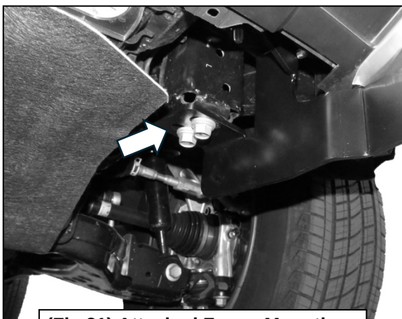
(Fig 21) Attached Frame Mounting Bracket to Driver/Left side
