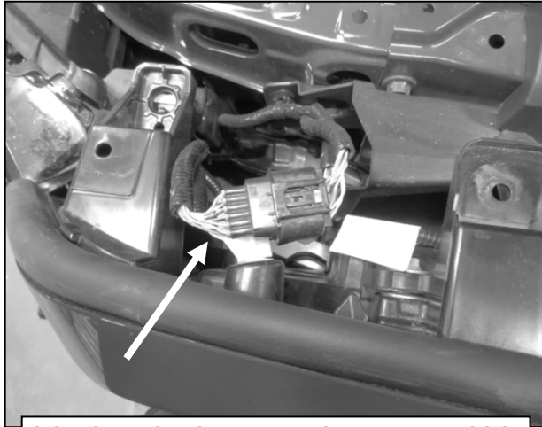
(Fig 3) Unplug harnesses (Passenger Side)
