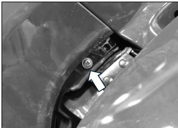
(Fig 5) Pull/Tug fender flare straight out to expose bolt. Remove bolt attaching fascia to fender. Repeat to passenger side.
