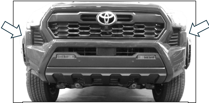
(Fig 8) With the top, bottom, and sides unclipped and unbolted, gently pull straight out on the sides (arrows) to take off the front clip.
