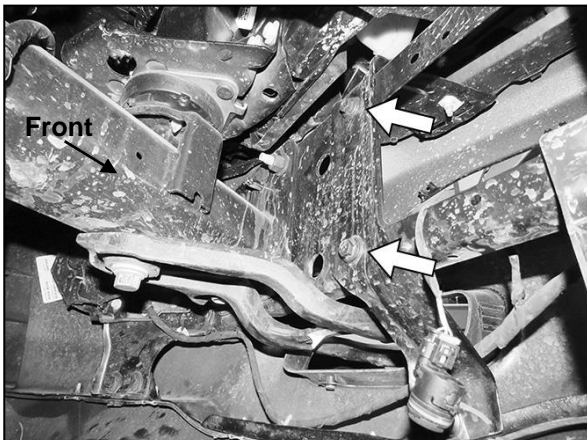
(Fig 3) Remove the (2) inner bumper bracket bolts (arrows). Driver/left side pictured from behind bumper
