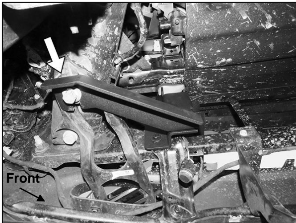
(Fig 11) Slide driver/left Support Bracket between tow hook (or spacer on bottom of frame) and body bolt
