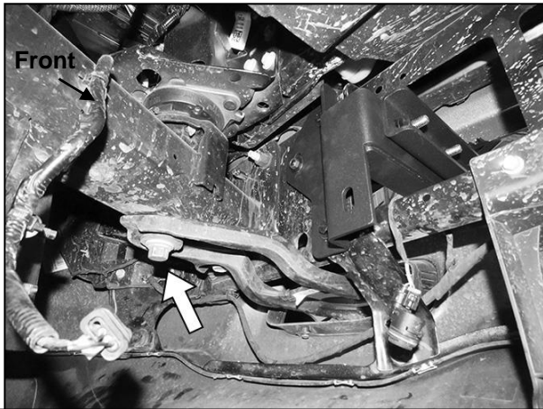
(Fig 9) Loosen but do not remove body mount bolt (arrow). Model with tow hook pictured
