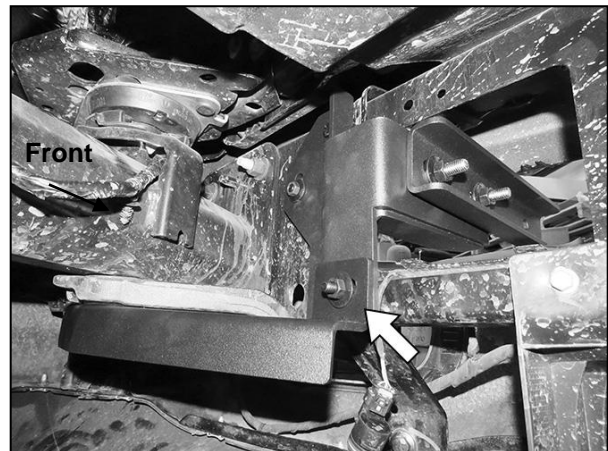
(Fig 12) Attach bent end of Support Bracket to back of Frame Bracket (arrow)
