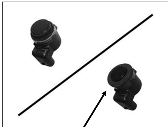
(Fig 17) Remove silicone seal from sensor. Slide large Seal over end of sensor (arrow)
