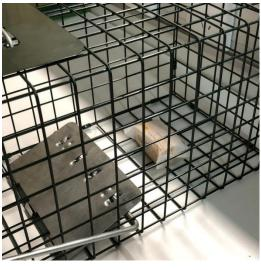
Step 4. Release the hook then the trap setting is finished. When an animal touches the plate in the cage the door will be triggered to close.
