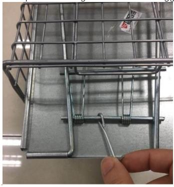
Step 5. How to release the animal the trap catches: Repeat Step 1-3 to set the hook on the wire to keep the door opening and release the animal.
