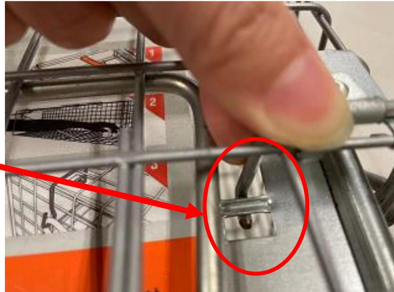
Step 4: Release the safety latch then the trap setting is finished.
