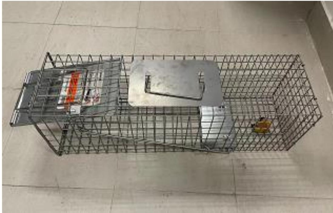
Step 3: Pull the door up to the top and latch hook through trap door until the trigger settled.
