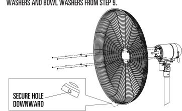
STEP 11 ASSEMBLE FAN BLADE ONTO MOTOR SHAFT BY TIGHTENING TWO SCREWS FROM BLADE. MAKE SURE THE SCREWS ARE
