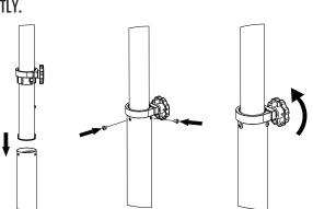
MOUNT THE FAN HEAD NOTO THE EXTENSION PIPE BY TIGHTENING THE SCREWS, WASHER AND NUTS. THE SCREWS, WAHSER AND NUTS STOCKED IN THE MOTOR BOX.
