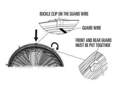
SECURE THE ASSEMBLY OF FRONT GUARD AND REAR GUARD BY TIGHTENING ONE SCREW M3\*10, TWO START WASHER  $\varphi$ 3 and one hexangular nut m3.
