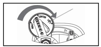
The switch rotates clockwise 360° to adjust the spray Angle .
