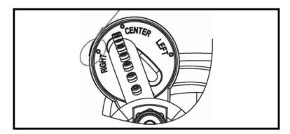
There are four spraying modes of the product, respectively **Right, Center, Left**, **and Full**, Turn the indicator to the desired spray pattern.
