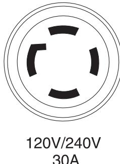
Use this receptacle to operate 120 Volt AC, 60 Hz, single phase loads requiring up to 3600 watts (3.6 kW) of power at 30 Amps or 240 Volt AC, 60 Hz, single phase loads requiring up to 7200 watts (7.2 kW) of power at 30 Amps. The outlet is protected by two 30 Amp push-to-reset circuit breakers.
