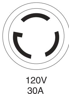
Use this receptacle to operate 120 Volt AC, 60 Hz, single phase loads requiring up to 3600 watts (3.6 kW) of power at 30 Amps. The outlet is protected by a 30 Amp push-to-reset circuit breaker.
