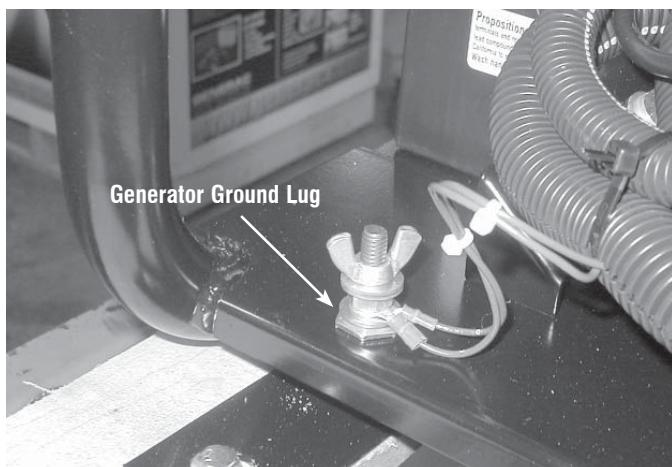
**Proper grounding of the generator will help prevent electrical shock** in the event of a ground fault condition in the generator or in connected electrical devices. Proper grounding also helps dissipate static electricity, which often builds up in ungrounded devices.
