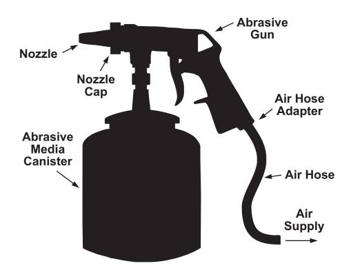
**WARNING:** Never open Abrasive Media Canister when air compressor is attached.
