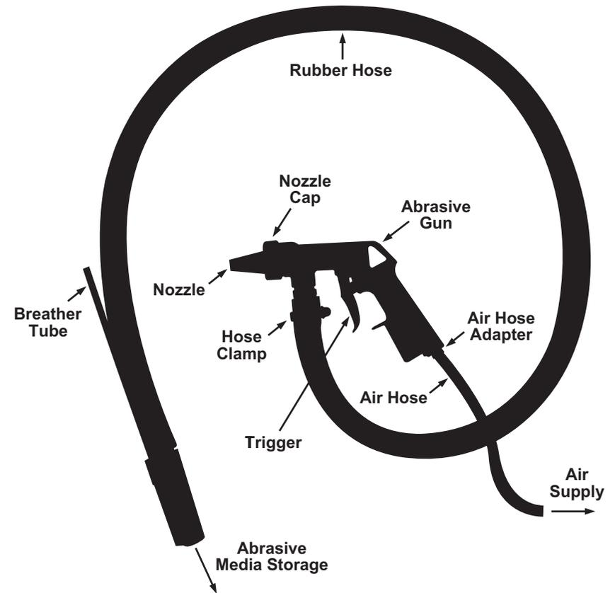
**NOTE:** Nozzle may become worn with time and need to be replaced. To replace, twist off Nozzle Cap and remove Nozzle. Attach new Nozzle and secure by twisting Nozzle Cap until securely tightened.
