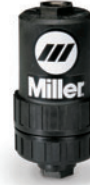
In-Line Air Filter Kit #228926 Mounts to the back of the AirForce™ 250ci, 500i and 700i. Includes male and female 1/4 inch NPT quick disconnect fittings and hose for easy on/off connection. The replaceable filter element filters to .85 microns.
