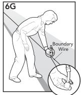
9. To test the run-through prevention feature, walk towards the Boundary Wire. The Receiver Collar should tone and the Test Light should flash brighter as you enter the run-through area (**6G**). If you are satisfied that your system is functioning properly, you are ready to start burying the Boundary Wire. If the Receiver Collar did not tone or the Test Light did not flash, see the "Troubleshooting" section.
