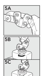
If the Receiver LED Indicator Light is flashing every 4 to 5 seconds, battery replacement is required. Remove the old battery from the Receiver Collar. Discharge all power by holding the correction level button down until the LED is no longer illuminated. Replace with a new battery.
