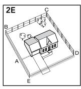
twist the wires from A back to the Fence Transmitter. See the "Install the Boundary Wire" section for more information on attaching the wire to a fence.
