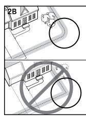
Sample 2 (2E): Perimeter **Loop Using Existing Fence** (Single Loop) This layout allows you to include your existing fence as part of your layout and keep your pet from jumping out or digging under your existing fence. It reduces the amount of wire which will need to be buried. From the Fence Transmitter, run the wire to A, A to B, B to C, C to D, D to E, E to A,
