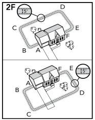
Sample 3 (2F): Front or Back Yard Only (Double Loop) From the Fence Transmitter, run the wire to A, A to B, B to C, C to D, D to E, E to F, make a U-turn and follow your path all the way back to A, keeping the wire separated at least 5 feet. Twist the wire from A back to the Fence Transmitter.
