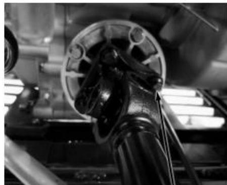
4 Bolts of front knuckle connected with the engine
