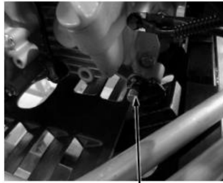
2 Bolts and Nuts of lower engine hanger
