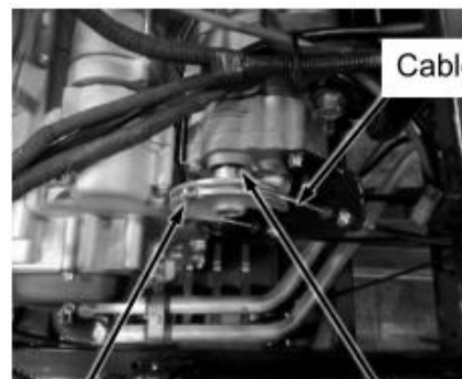
Shifting Anchor Plate Bolt
