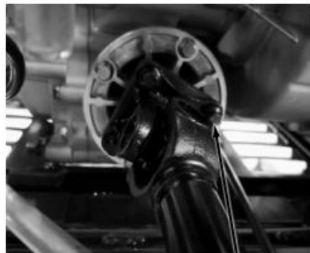
4 Bolts of front kunckle connected with the engine
