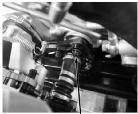
4 Bolts of rear kunckle connected with the engine
