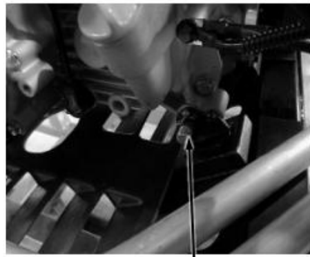
2 Bolts and Nuts of lower engine hanger
