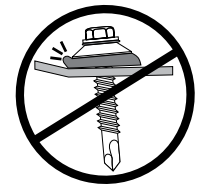
INCORRECT Non-perpendicular. Figure 8c
