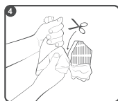
4 Cut corner and squeeze material to fill hole
