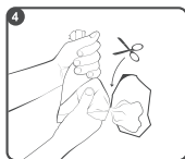
4 Cut corner and squeeze material over first coat
