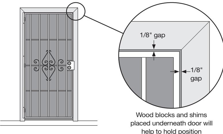
Position door/hinge-side jamb assembly (**A**) in front of opening. Allow for a 1/8" gap between the lock-side edge of door and inside edge of your mounting surface, as well as a 1/8" gap between the top edge of door frame, (not the thin fly strap welded to the edge of the door frame in select models) and bottom edge of your mounting surface. Make certain the assembly is plumb.
