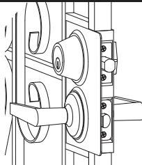
Install your choice of locksets with 2-3/8" backset (sold separately). Fully extend the lock bolts into the "locked" position.
