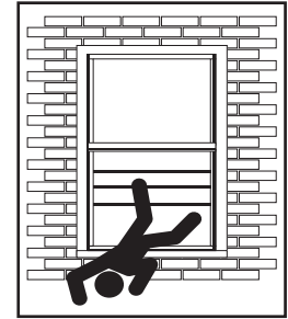
Installed to low
