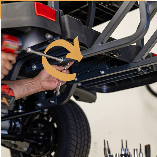
Use included fasteners to secure the caddy to the MEV 2X frame
