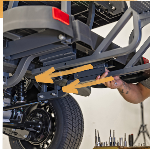
Align Caddy Frame to attachment points
