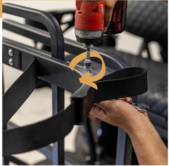
Secure bag holder, tighten to 18 lb/ft
