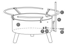
5. Place the adjustable tube [J] over the top of the swing grill stand [K], then insert the swing grill [L] into the swing grill stand. Use the lock ring [I] to adjust the height of the swing grill.
