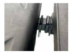
Step 5: Slide on the metal plate with the bend facing the front of your vehicle. Please make sure the bent portion is over the lip of your vehicle's hitch adapter. Once this is in place add the washer, lock washer and nut. Tighten the nut with a wrench until the bolt is securely fastened and there is no movement of your tank.
