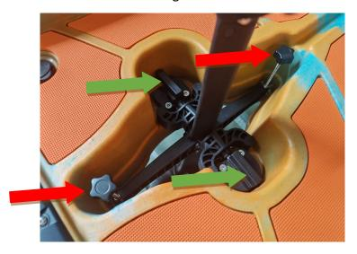
Once this is complete and the drive is secure, there should be no side to side or forward and back motion in the drive. You'll now add the splash guards around the drive. Gently push these into place until they are flush with the deck.
