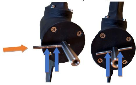
Once this is in place, put the propeller onto the drive. You will need to gently rotate the propeller until it drops into place and locks over the shaft pin. To test you have this right, move the pedals and the propeller should now start to spin. Open the little plastic bag with the screw and lock washer. Place the lock washer onto the screw and screw this into place to secure the propeller to the drive.
