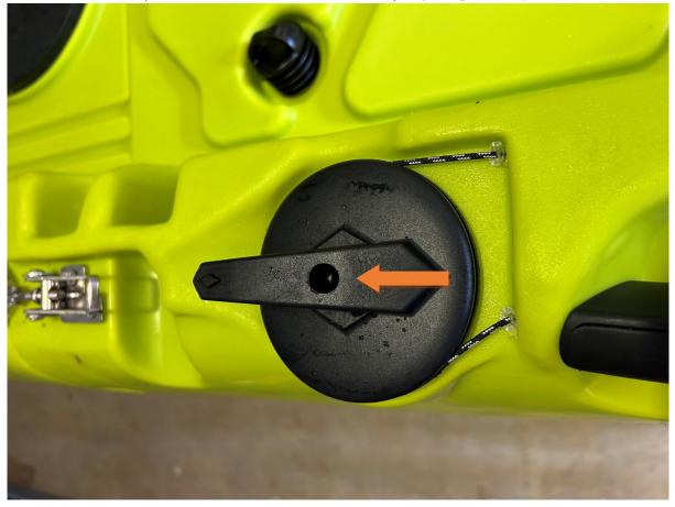
Next, ensure your rudder is untangled and the lines run free when taking it out of the cargo area. Put the pin of the rudder through the rear hole in the kayak. Check that the raising and lowering of the rudder operates smoothly. Next put in the rudder security pin (orange arrow) through the hole at the bottom of the rudder pin.
