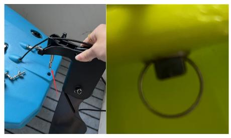
Next unwind the butterfly nuts and put them through the plastic holes on either side of the rudder and righten the butterfly nuts again.
