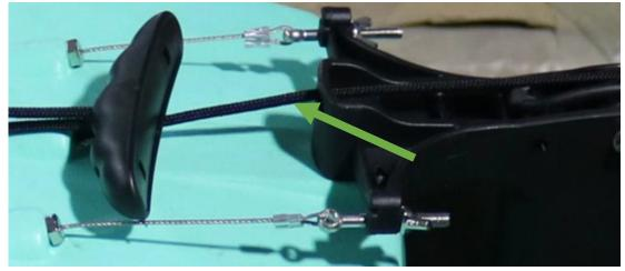
Next grab hold of the rudder steering handle on the left side of the kayak near where the seat would be located. Pull the rudder handle all the way left and then all the way right, to ensure the rudder is tracking correctly, adjust the butterfly nuts as needed. Leave the rudder steering in the approximate centre spot. The steering wires should have a little bit of slack for ease of turning and to ensure minimal wear and tear where they enter the kayak.
