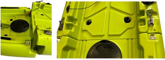
Next close the latches on both sides. The latches should be set correctly for your kayak, but if you find you're having to force it <u>then stop.</u> Adjust the nut (orange arrow) to get a firm lock closure, but not without forcing it. If it's too loose then adjust the nut accordingly to get a good firm fit. Forcing the latch closed for an overly tight fit can damage the screws unnecessarily (blue arrow) on the adjoining catch.
