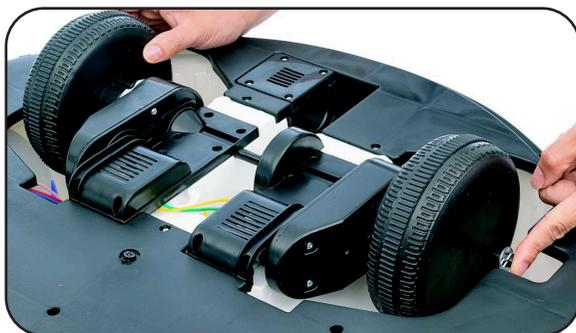
3. Slide axle to either side to properly insert rear wheel. Ensure the wheels are aligned with sprocket.
