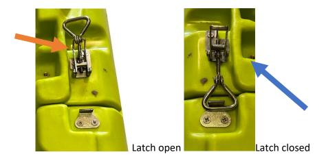
Step 4: Roll the kayak on its side and close the two latches underneath.
