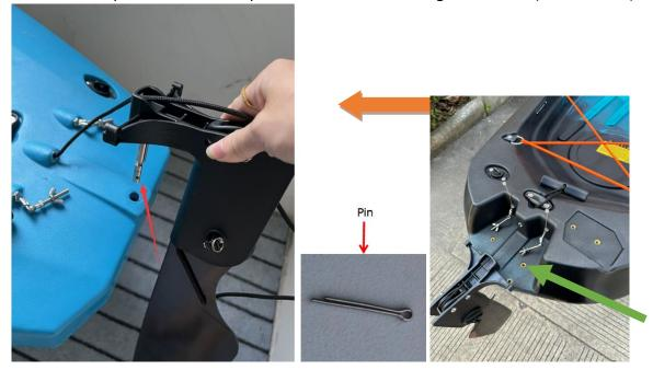
Next unwind the butterfly nuts and put them through the plastic holes on either side of the
