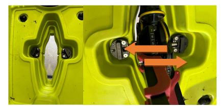
Note sometimes it requires pulling the pedals firmly to the left and right (orange arrows) each time when inserting the drive for the pins to lock in place. However you do need to keep this in mind when beaching the kayak, by always pushing forward on one of the pedals to ensure the flaps are flared and <u>being careful</u> when dragging the kayak up the beach.
