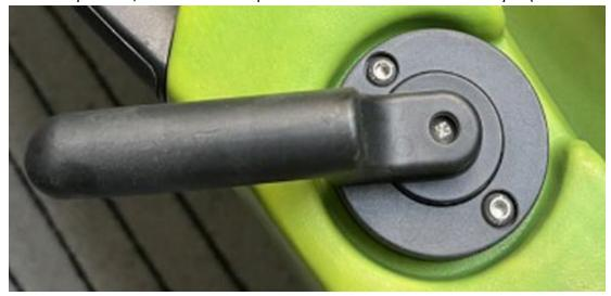
Start by ensuring that your rudder steering handle is in a neutral position with the handle parallel to the centre line of the kayak (orange arrow).
