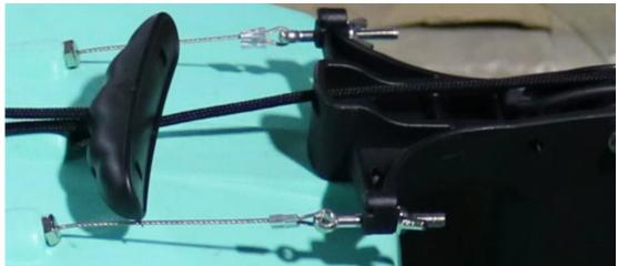
Next grab hold of the rudder steering handle on the left side of the kayak near where the seat would be located. Pull the rudder handle all the way left and then all the way right, to ensure the rudder is tracking correctly, adjust the butterfly nuts (Orange arrow) as needed. Leave the rudder steering in the approximate centre spot. The steering wires should have a little bit of slack for ease of turning and to ensure minimal wear and tear where they enter the kayak.
