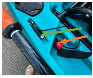
The rope with the red ball (Orange arrow) on the right of your seat controls the raising and lowering of the rudder. TO lock it in place pull the rope backwards to "cleat" (Green arrow) it into place in the up position. To lower it, uncleat the rope and let it run free.
