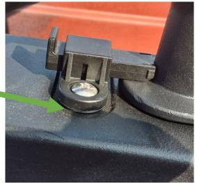
Note there is a shim under the propeller drive lock. If you find there is some side to side shift when pedalling you can remove the shim (Green Arrow) underneath to provide a tighter fit.
