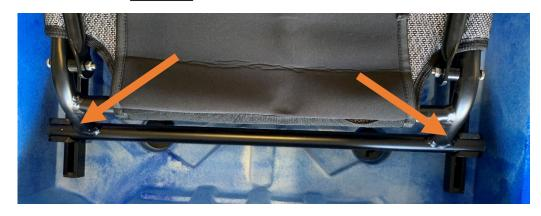
Lastly connect and secure the two side straps which hold the back of the seat upwards. Secure this in a slightly off of 90 degree upright position, this can be further adjusted once you're on the water. Also remember to take your allen wrench on your first couple of outings in case you want to further adjust your seat location.
