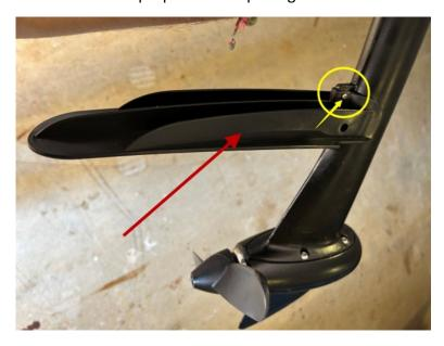
After you have installed the pedal drive, next is to secure the cup holder and pedal drive pod cover. This should be inserted pushing the front down (Orange Arrow) towards the pedal drive and forward firmly. This may require some force to have it fit snuggly to provide an optimal seal around the pedal drive, once in place clip the bungy cables on each side over.
