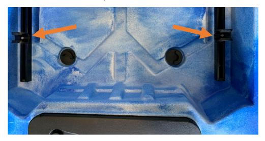
Sit the back bar of the seat on top of the brackets, but don't pop them in yet. Screw the front of the seat into the two front slider receivers.
