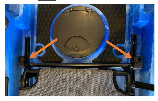
Step 3: Put the four seat raisers on the seat bars. Ensure that each of the feet is pointing out from the chair and not in under the chair. Secure each screw into their respective rail sliders.
