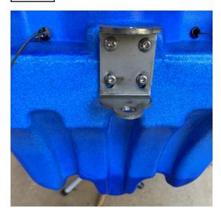
Next, ensure your rudder is untangled and the lines run free. Put the pin of the rudder through the rudder bracket holes. Check that the raising and lowering of the rudder operates smoothly. Next put in the rudder security pin through the hole at the bottom of the rudder pin. Using a knife, screwdriver or pliers open the security pin ends (green arrow) to prevent losing the rudder, through the pin popping out.
