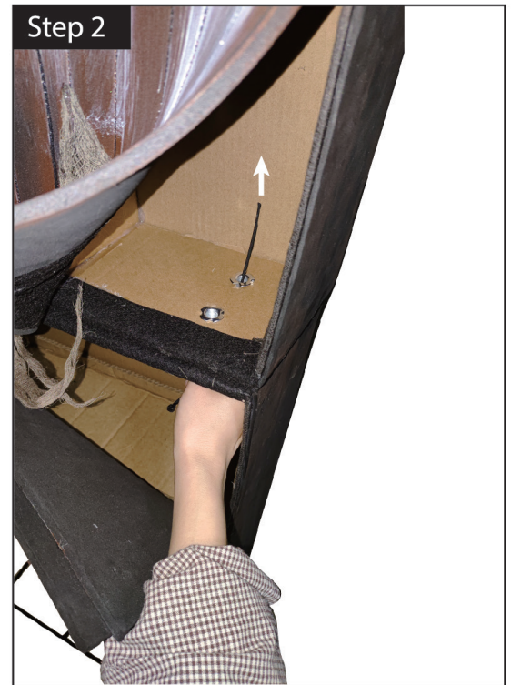
Step 2- Open the right corner of the two sections of the lid. Thread the longer zip tie through the holes in the bottom section to the holes in the top section. Repeat the same step on the left side.
