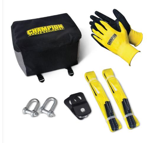
Champion's ATV winch rigging kit contains all the basic tools you need for recovering your ATV or other winching operations. The soft storage case contains a pair (2) of 1.4-ton-rated D-shackles, two (2) 8,800-lb.-rated tree anchor or tow straps, one (1) 8,000-lb.-rated snatch block, and a pair (2) of utility gloves.
