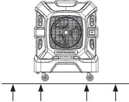
Position the cooler on a level surface while in use. Lock the caster wheels.
