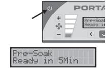
Pressing the power button on the cooler will begin a pre-soak function for the media. During this pre-soak, the fan will run at low speed (the LCD screen will display a countdown timer).
