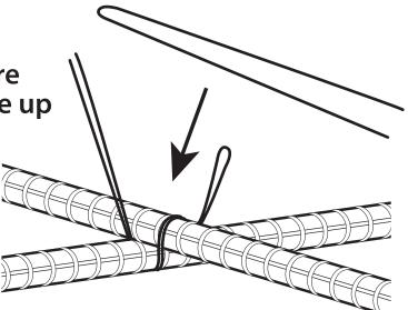
2 Loop both ends around rebar tie tool and spin until the wire is tight and holds joint securely.
