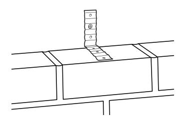
3 Set next coarse of bricks over the tie. The mortar will secure the tie.
