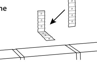
Attach tie to structure with nails or screws
