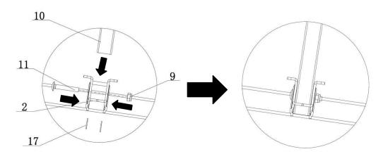
Here it is necessary to reach a torque of 50Nm so that the square tube does not shake.
