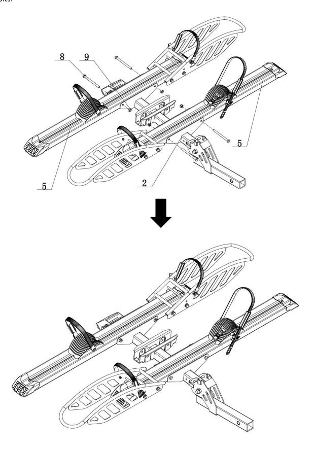
**Step 4**: Insert Middle Support Tube (10) into the base of Bottom Fixing Bracket (2), at the same time, insert the half round gasket (17) from the bottom up to the middle of the square tube and the bottom plate boss to separate, then fix them with M10x60 (11) and M10 Lock Nut (9).
