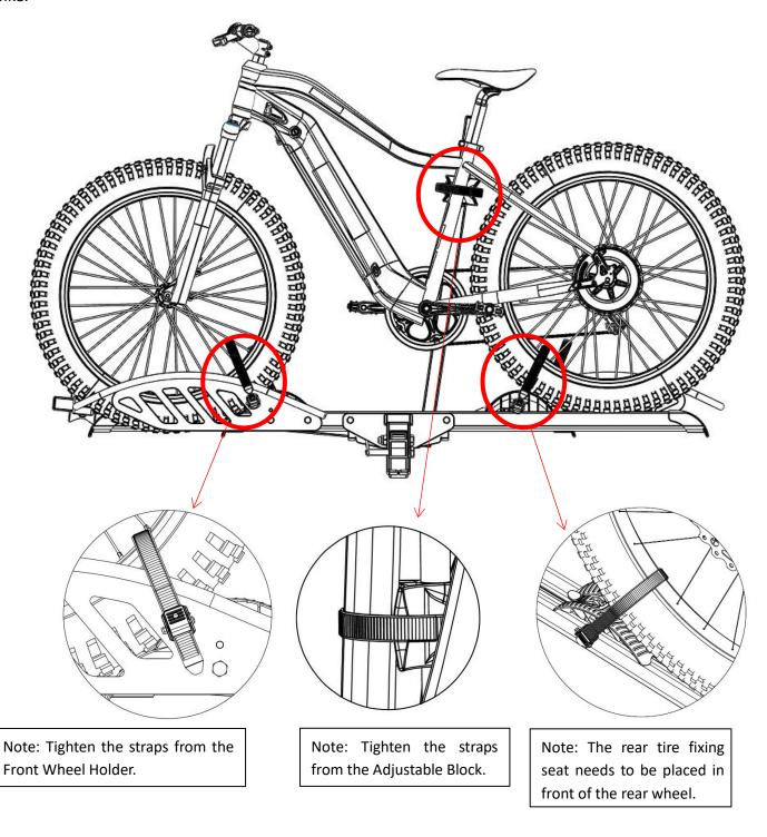
When the bike's tire is against the wheel cradle, press down the button on the wheel cradle to secure it firmly.
