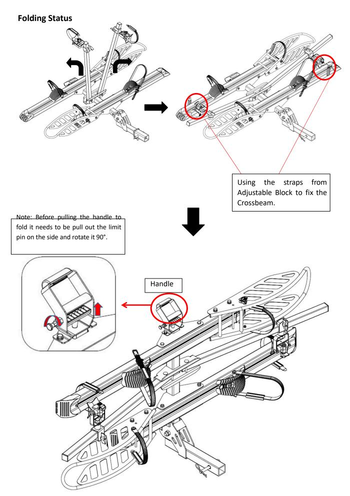
Pull the handle in the direction the arrow shows to fold the bike rack vertically, or to unfold it so it sits flat. The bike rack will automatically stop when it reaches a fixed position
