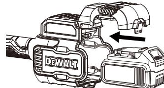
**! WARNING:** To avoid serious personal injury, always remove the battery pack and keep hands clear of the lock-out button when carrying or transporting the tool.
