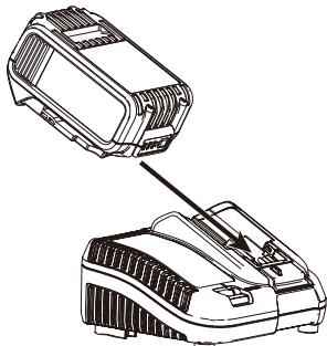
2. Insert the battery pack into the charger, making sure the battery pack is fully seated in the charger. The red (charging) light will blink continuously indicating that the charging process has started.
