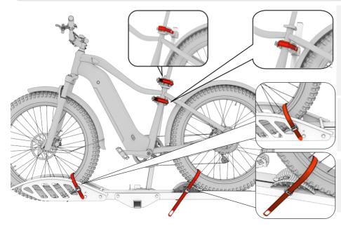
Note: Use the ratchet wheel strap to fix and tighten the seat/middle tube of the bike. Buyer should take full responsibility if any damage is caused by the lack of securing the seat tube well and being clamped in a location other than the seat/middle tube.
