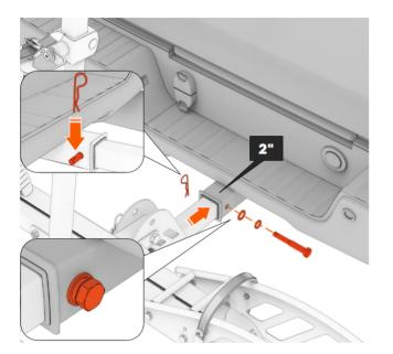
Align the holes of the folding tube with the holes on the vehicle's **2" hitch receiver**, then connect the two parts as shown below. Place a **M16 shockproof bolt (10)**, through the  $\phi$ **16 Spring Washer (11)**,  $\phi$ **16 Flat Washer (12)** and the aligned holes. Screw the bolt in place by Monkey Wrench (Not included) and secure it with the  $\varphi$ 3.8 pin (13), making sure to place the pin through the holes on the bolt.
