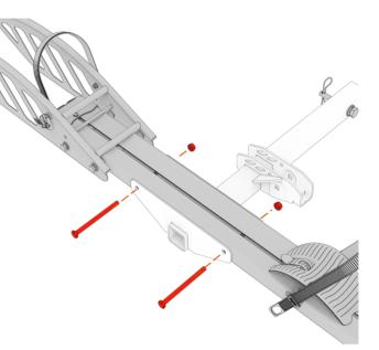
Put the holes of the **Front Wheel Holder (3)** and the **Beam** Assembly (1) aligned, install 4pcs M10\*25 Outer Hexagon Bolt Kits (2) and tighten them. Place the components assembled in steps 1 above into the **Bottom Fixing Bracket (6)**, align the holes, install 2pcs **M10 Long Outer Hexagon Bolts (4)** and 2pcs **M10 Lock Nuts (5)**, and tighten the bolts.
