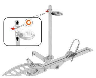
Insert the **Support Rod (7)** into the **Bottom Fixing Bracket (6)**, align the holes, place the **Semicircle Plates (15)** on both sides of **Support Rod (7)**, install the **M10 Low Square Neck Bolt (8)** and the **M10 Lock Nut (5)**, and tighten them until the support rod does not move. Insert the adjustable **Connecting Block (9)** into the **Support Rod** (7), and properly tighten the knob so that it does not slide down.
