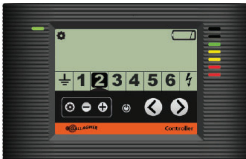
Controller showing zone 2 with a low battery
