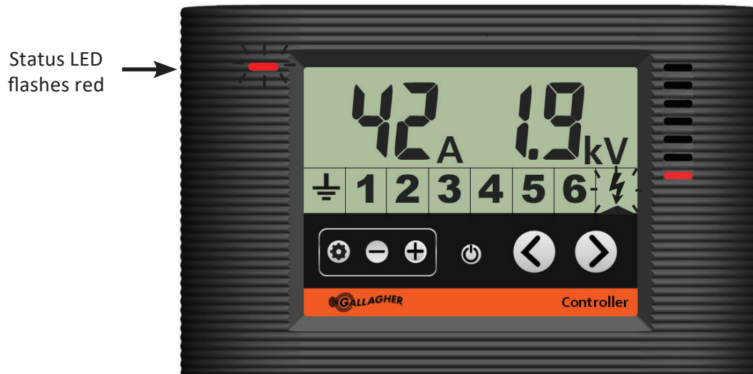
Controller showing the energizer in current alarm
