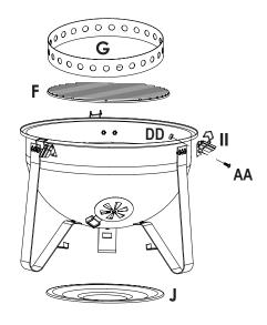
**STEP 3:** Attach grid holder 6 x (N) to the middle bowl (C) using bolts 6 x (CC) and nuts 6 x (FF). Attach door (I) to the middle bowl (C).
