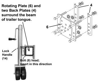
Note: Pull up on the Lock Handle (14) to disengage the Rotating Plate (6) so it can be moved to vertical, or horizontal position.
